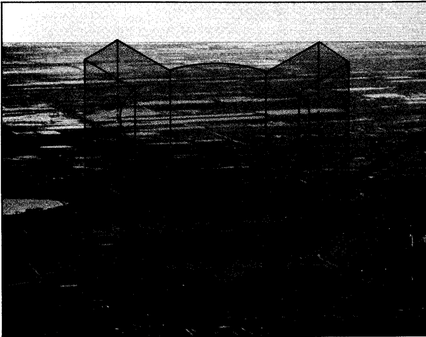
Figure 2-31. A control zone extends from the surface up to the base of the continental control area at 14,500 feet MSL. If a particular control zone is not under the continental control area, it has no upper limit.
