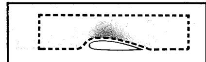
Figure 1-15. Air flowing over the top of an airfoil reaches the trailing edge in the same amount of time as air flowing along the relatively flat bottom. Since both the upper and lower surfaces pass through a block of air at the same speed, the air flowing over the curved upper surface travels farther. This means it must go faster, resulting in lower pressure above the airfoil than below.
